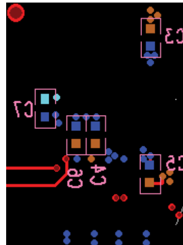
Figure 55. Bottom Layer decoupling
